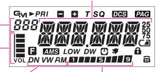
S Meter: Displays the received signal strength PO Meter: Displays the transmit power level
